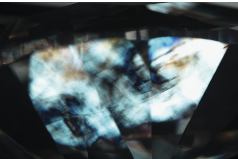
Figure 3. Left: Mottled strain patterns with high interference colors observed under cross-polarized light. Photomicrograph by Christopher Vendrell; field of view 7.19 mm. Right: DiamondView fluorescence image showing crystal growth patterns and the blue color commonly observed in type IaAB diamonds.
