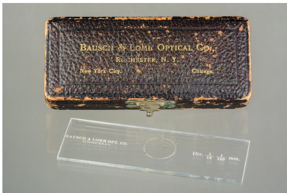
Figure 22. A microscope calibration slide, such as the one manufactured by Bausch and Lomb Optical Co., can be used to determine the actual field of view of an image taken through the microscope. Photo by Robison McMurtry.
