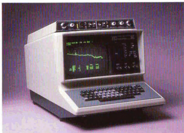
Figure 12. The ND 65B Multi Channel Analyzer (MCA) shown here is a pulse-height analyzer that converts electrical signals from either a NaI or a Ge(Li) detector into useful information such as the type and quantity of radioactive nuclides present in a gemstone. Courtesy of Nuclear Data, Inc., Schaumburg, IL.
