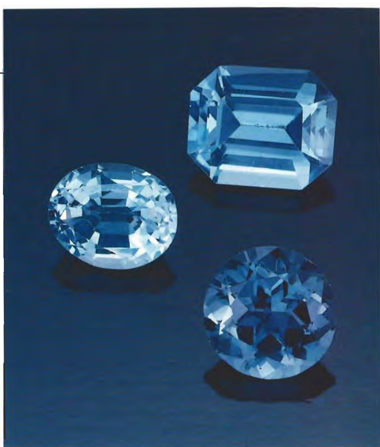
Figure 10. Far more topaz than any other gem material is being irradiated in laboratory facilities. The American Gem Trade Association (Willett, 1987) has estimated that 6,000 kg (30 million carats) of topaz are irradiated annually, 40% of this total in the U.S. Each of the stones shown here was treated by a different method (from lightest to darkest): linac-treated "Sky Blue," combination reactor- and linac-treated "California Blue," and reactor-treated "London Blue." Photo © Tino Hammid.
