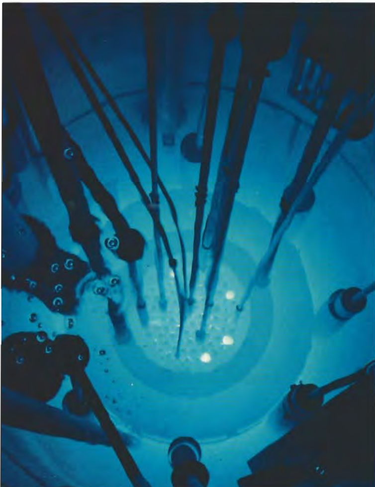
Figure 9. This photo was taken looking down into the pool of a TRIGA nuclear research reactor. The bluish glow seen here and in the gamma-ray facility in figure 6 is called Cherenkov radiation. It is produced by gamma rays interacting with the electrons of the water molecules and causing them to very briefly travel faster than light does in water. The electrons must slow down, and consequently lose energy by emitting photons of light. Photo courtesy of General Atomics, San Diego, CA.
