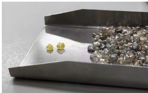
Figure 8. Two yellow cuboctahedral diamonds separated during recovery sorting in the processing plant at the Lomonosov mine. Photo by Karen Smit.
