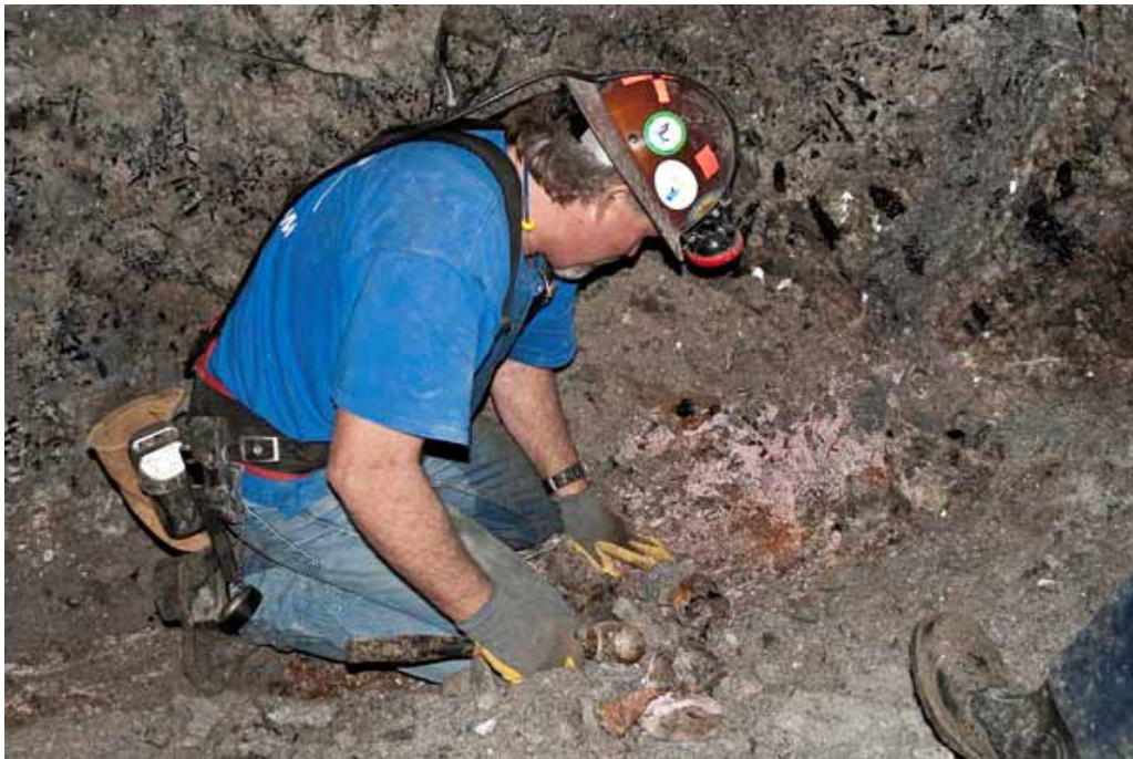
Figure DD-1. Daron Fisler inspects a new spodumene zone along the footwall of the pegmatite.
