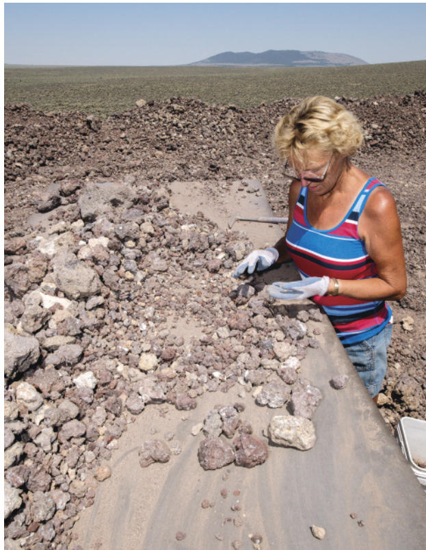
Figure 18. Sunstone Butte co-owner Tammy Moreau taps on the back of a piece of volcanic matrix with a small hammer to release feldspar phenocrysts. Photo by Robert Weldon.
