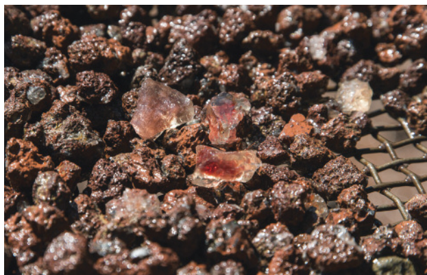
Figure 9. During screening, sparks of red to pink rough sunstone glitter in the sun among pea-sized chunks of vesicular basalt. Photo by Robert Weldon.
