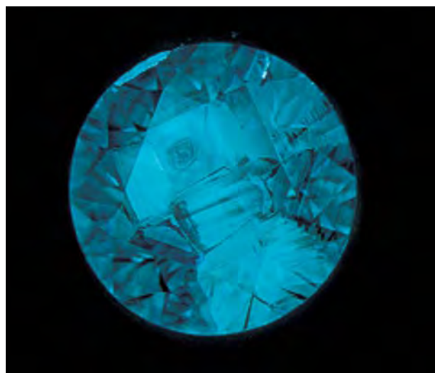
Figure 18. The cathodoluminescence of this 0.27 ct blue synthetic diamond reveals the distinctive arrangement of internal growth sectors. Photo by S. Muhlmeister and C. M. Breeding.
