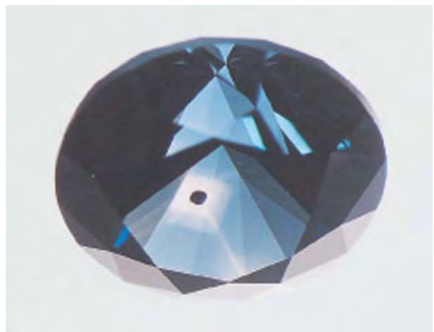
Figure 16. Like nitrogen, boron becomes concentrated in some internal sectors and not in others during crystal growth, leading to these distinctive patterns of blue and colorless zones separated by sharp boundaries. Photomicrograph by J.E. Shigley; magnified 20x.
