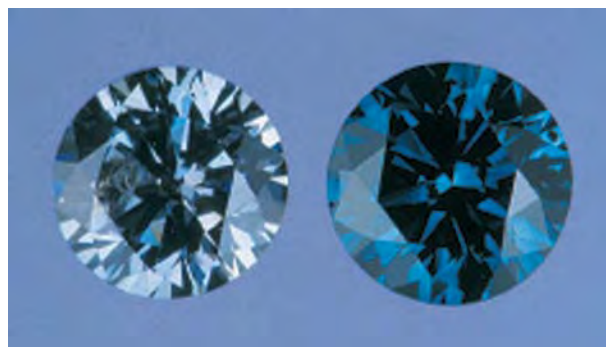
Figure 13. Different boron contents are responsible for the variation in color saturation in the blue lab-grown diamonds (here, 0.22 and 0.27 ct). Photo by Maha Tannous.
