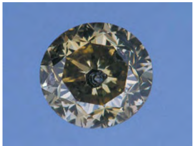
Figure 9. When examined with a prism spectroscope, the spectrum of this 0.34 ct green-yellow synthetic diamond (with a large metallic inclusion near the culet) exhibited a weak 595 nm absorption band, which indicated that it had been irradiated and heated to change its color. Photo by Maha Tannous.
