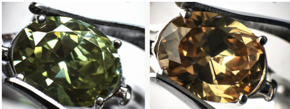
Figure 17. This synthetic cubic zirconia imitation of peridot, with an estimated weight of 4.50 ct, is shown in daylight (left) and incandescent light (right). Photos by Igor Iemelianov; field of view 13.20 mm.
