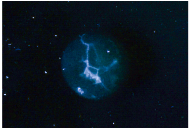
Figure 26. Some lines, along with the cavity, fluoresce white when exposed to long-wave UV radiation, indicating the presence of filling material. Photo by Wen Han.
