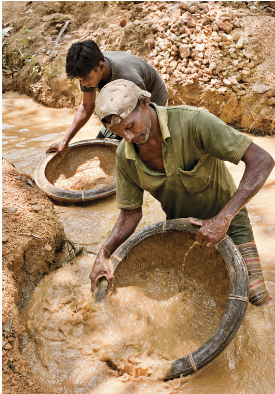
Figure 9. Washing sediments to recover fragments of gems in 2011 near Ratnapura, Sri Lanka. Photo by Vincent Pardieu.
