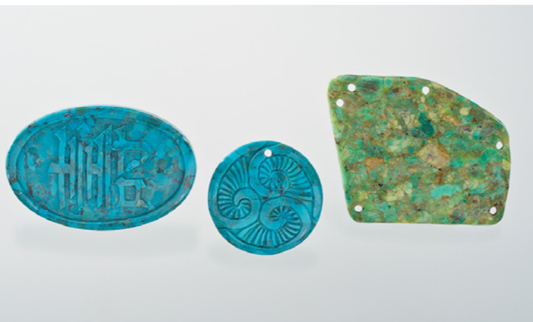
Figure 25. The demand for turquoise is so strong that low-quality material is being treated by polymer impregnation and pressed into a composite material to make it salable. The treatment is sometimes so extensive that the gemological properties are altered. These carvings, 3.0–6.0 cm wide, are courtesy of Silver Express; photo by Robert Weldon.
