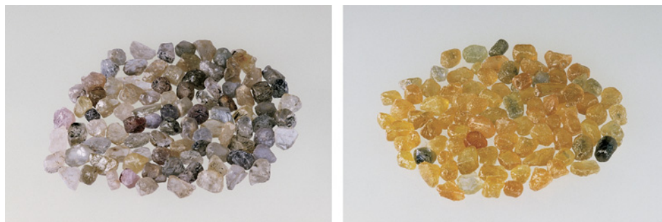
Figure 11. As these before-and-after images illustrate, beryllium diffusion can produce profound color alterations in corundum, here turning 1–2 ct light blue sapphires to intense yellow. Photos by Maha Tannous.
