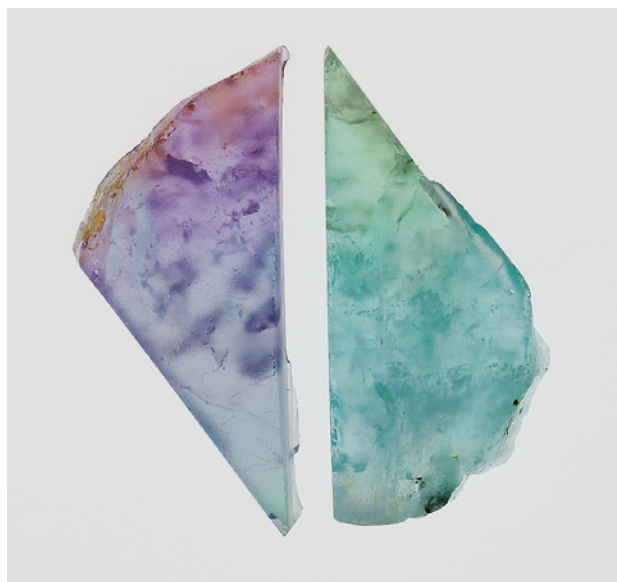
Figure 8. This copper-bearing tourmaline from Mozambique was cut in half, and the piece on the right ( 8 \times 20\text{ mm} ) was then heat treated. Photo by C. D. Mengason.
