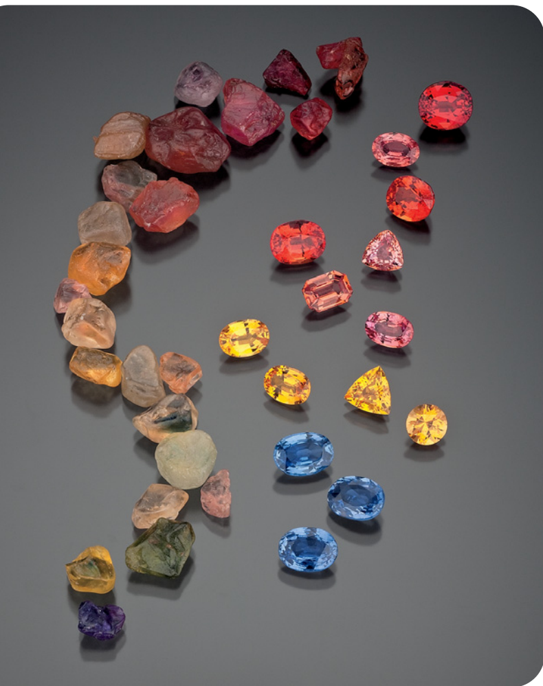
Figure 10. Almost every color of corundum can be affected in some way by beryllium diffusion, as illustrated by this large group of Be-diffused rough and faceted stones (1.03–8.53 ct). Photo by Robert Weldon.
