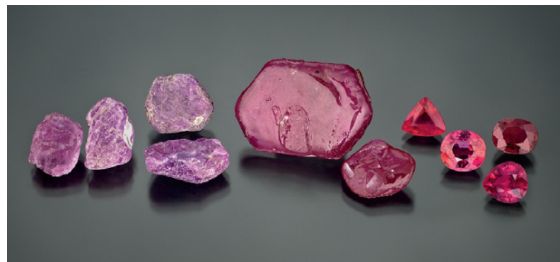
Figure 17. Filling ruby with a lead-based glass can change non-gem corundum (on left) to transparent, facetable rubies such as those on the right. The samples (2.13–39.17 ct) are courtesy of Hussain Rezayee and GIA; photo by Robert Weldon.
