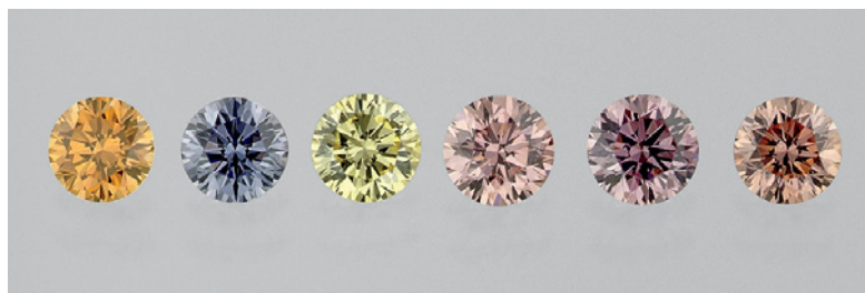
Figure 21. New coatings can turn diamonds virtually any color, as illustrated by these ~0.40 ct coated diamonds. Courtesy of Serenity Technologies; photo by C. D. Mengason.
