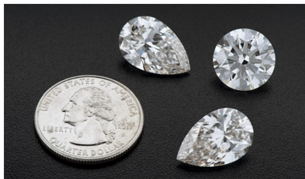
Figure 7. Three large CVD-grown diamonds submitted by Plasmability to GIA for scientific examination: A matching pair of pear-cut gems weighing 8.88 and 8.89 ct, as well as a 10.13 ct round brilliant. These American-grown diamonds are displayed with a U.S. quarter (24.26 mm diameter) for scale. Photo by Jian Xin (Jae) Liao.
