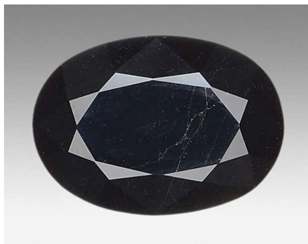
Figure 2. A 22.33 ct oval mixed-cut gadolinite exhibiting a very dark and almost opaque bodycolor and multiple fractures covering the surface. Photo by Shunsuke Nagai.
