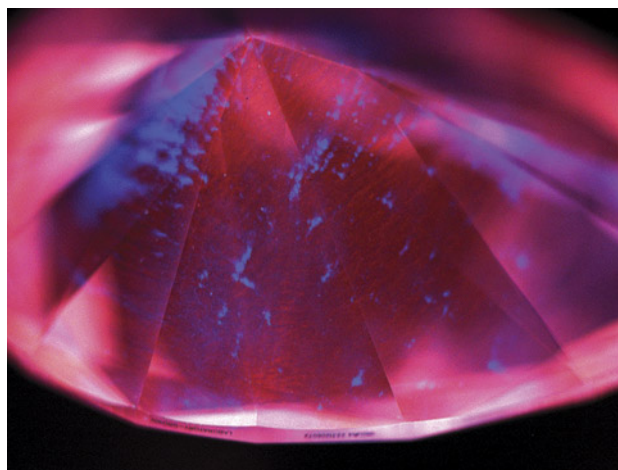
Figure 8. Representative deep-UV fluorescence image of a 2.90 ct CVD diamond from Plasmability, collected using the DiamondView. The image is dominated by red–orange fluorescence from NV^0 centers, a common feature for untreated CVD laboratory-grown diamonds, along with irregular blue fluorescing dislocation bundles. No growth layers were observed, indicating that it was produced through a single uninterrupted growth cycle. Image by Madelyn Dragone.
