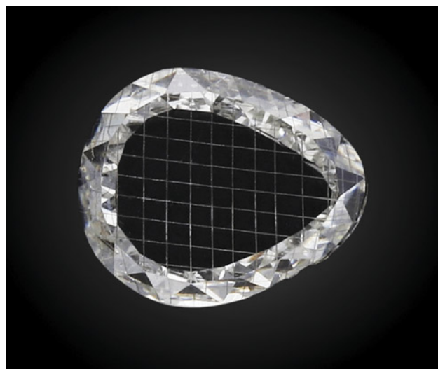
Figure 1. This 1.02 ct modified pear portrait-cut natural diamond has a checkered pattern on the flat pavilion, created using a laser. Photo by Gaurav Bera and Tejas Jhaveri; field of view 7.10 mm.
