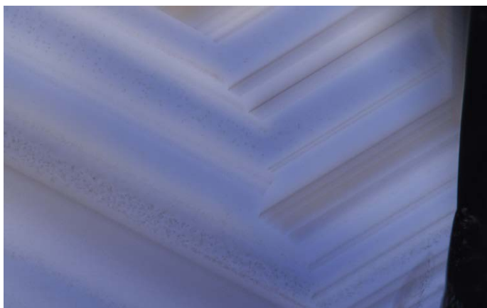
Figure 19: When correctly illuminated, the areas with highest particle density appear brownish in GIA reference sample 668841902. Diffused illumination. FOV 1.75 mm. Photo: V. Raynaud © GIA.
