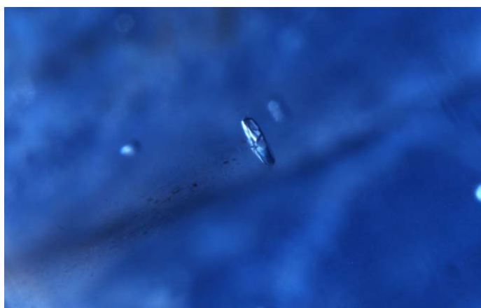
Figure 55: Elongated feldspar crystal with trail of particles in GIA reference sample 100322689774. Darkfield and fiber-optic illumination. FOV 1.3 mm. Photo: C. Khowpong © GIA.
