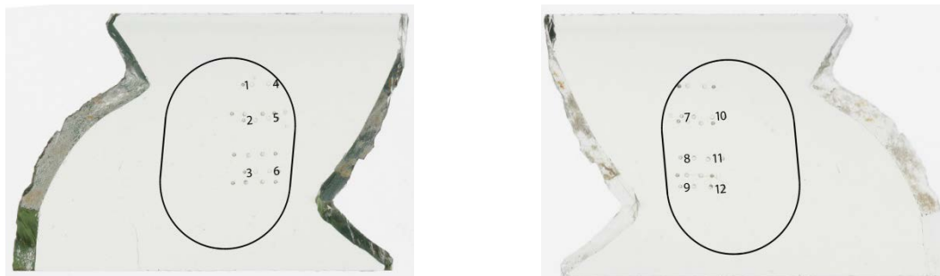
Figure 69: GIA reference sample #5040 showing the location of the 12 spots where LA-ICP-MS analysis was conducted on each side of the wafer. Field of view 3.00 mm. Photo: S. Engniwat © GIA.
