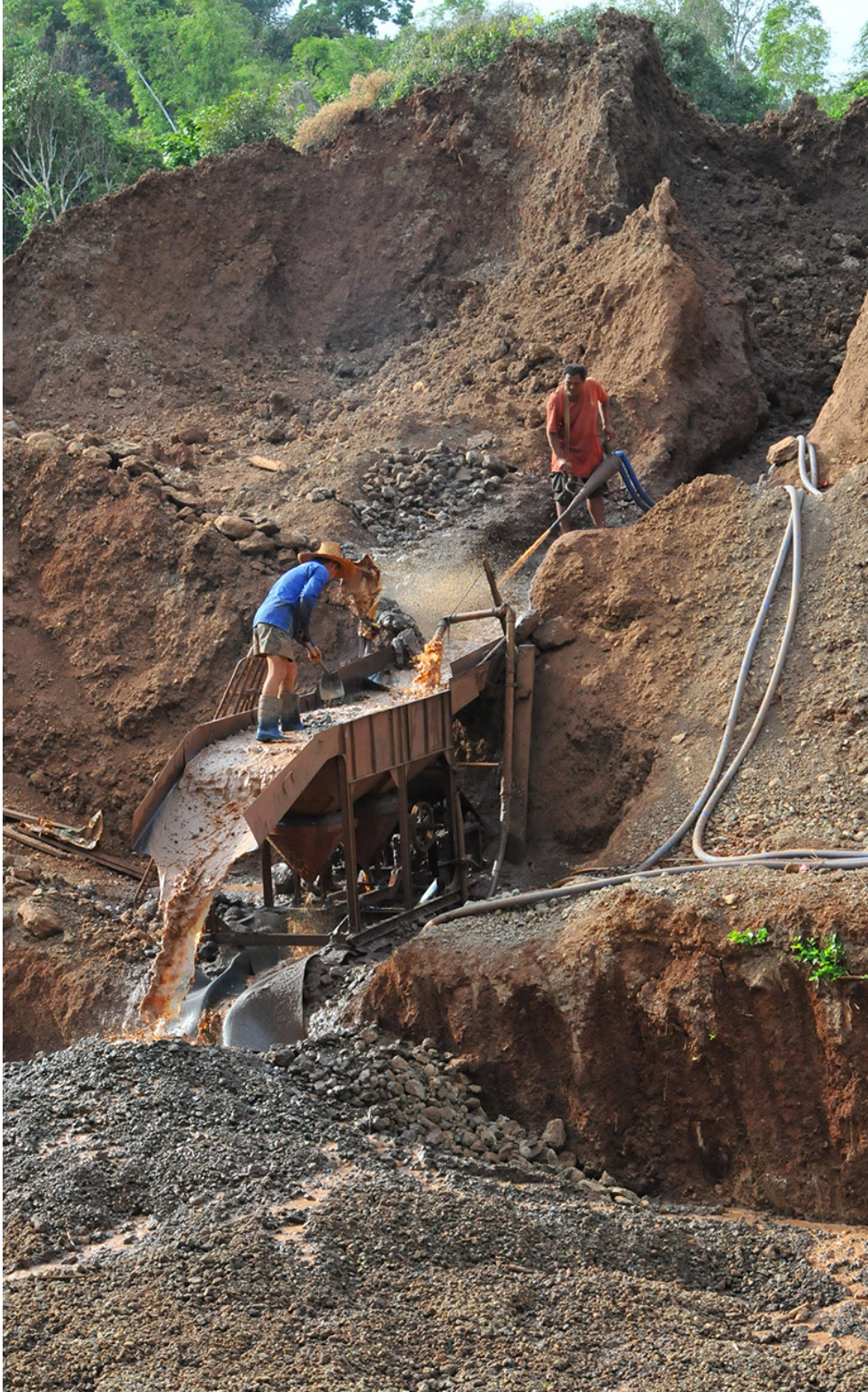
Figure 13: View of Mr. Wuyi's mine near Khao Ploy Waen. The material is washed from the pile on the right, through the jig in the center into the pit on the left side. Photo by Vincent Pardieu © GIA.
