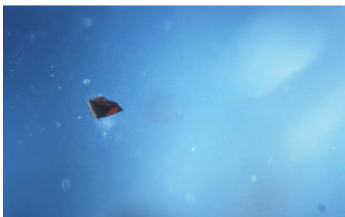
Figure 56: A brownish oryngy crystal (identified by Raman as pyrochlore using the RRUFF database as a reference) in GIA reference sample 668889302. Darkfield and fiber-optic illumination. FOV 0.7 mm. Photo: V. Raynaud © GIA.
