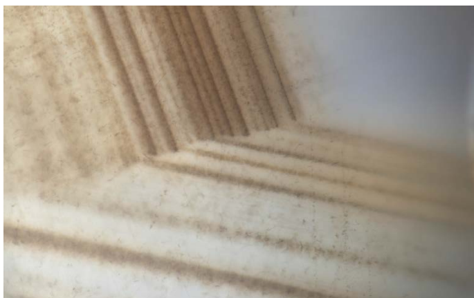
Figure 21: Under diffused illumination, the angular bands of brownish particles clearly contrast with the particle-free areas in GIA reference sample 668839802. FOV 1.2 mm. Photo: V. Raynaud © GIA.
