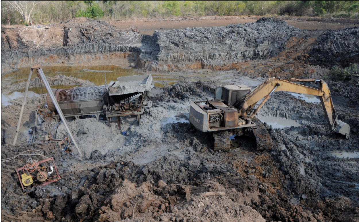
Figure 14: An excavator digging sapphire-bearing ground near Bang Kaja. The excavator dumps material in the jig's feed bucket, where it goes into the revolving screen. The washed gravels move towards the gravel pump (at the base of the tripod). Note the contrast between the gray marine clay and the red weathered basalt in the background. Photo by Wim Vertriest © GIA.
