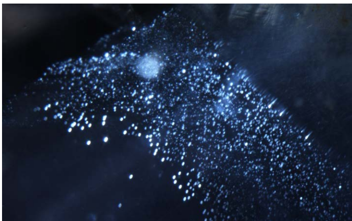
Figure 36: Reflective thin films in GIA reference sample 100322689757. Darkfield and fiber-optic illumination. FOV 2 mm. Photo: C. Khowpong © GIA.
