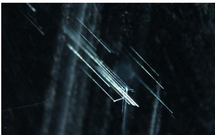
Figure 32: Intersecting needles in GIA reference sample 100305161405. Darkfield and fiber-optic illumination. FOV 2.7 mm. Photo: C. Khowpong © GIA.
