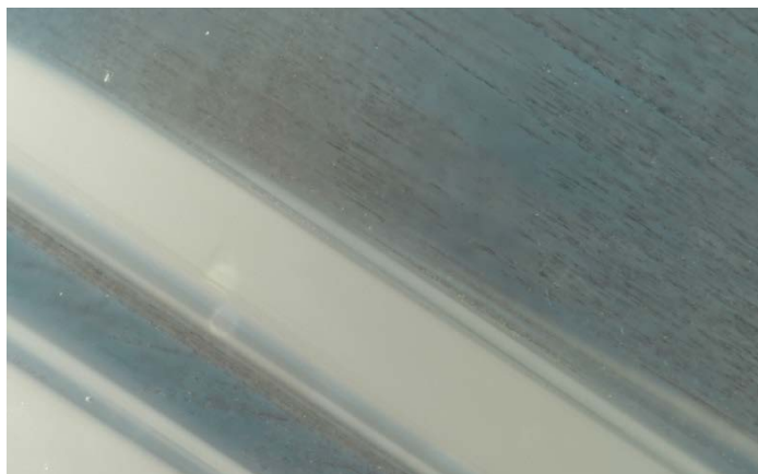
Figure 23: Under diffused illumination, bands of brownish particles clearly contrast with the particle-free areas in GIA reference sample 668839802. FOV 1.2 mm. Photo: V. Raynaud © GIA.
