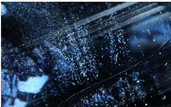
Figure 34: Irregular rutile needles and reflective fluid inclusions in GIA reference sample 100322689760. Darkfield and fiber-optic illumination. FOV 2.7 mm. Photo: C. Khowpong © GIA.
