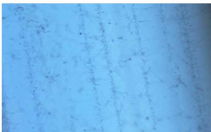
Figure 27: Platy brownish needles stand out under diffused illumination in GIA reference sample 100305161818. FOV 8.2 mm. Photo: V. Raynaud © GIA.
