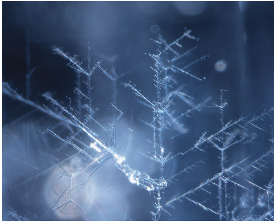
Figure 9. Unique hollow channels resembling rime ice in a 1.78 ct jeremejevite. The vertical direction of this photo corresponds to the c -axis of the stone. Photomicrograph by Makoto Miura; field of view 1.48 mm.
