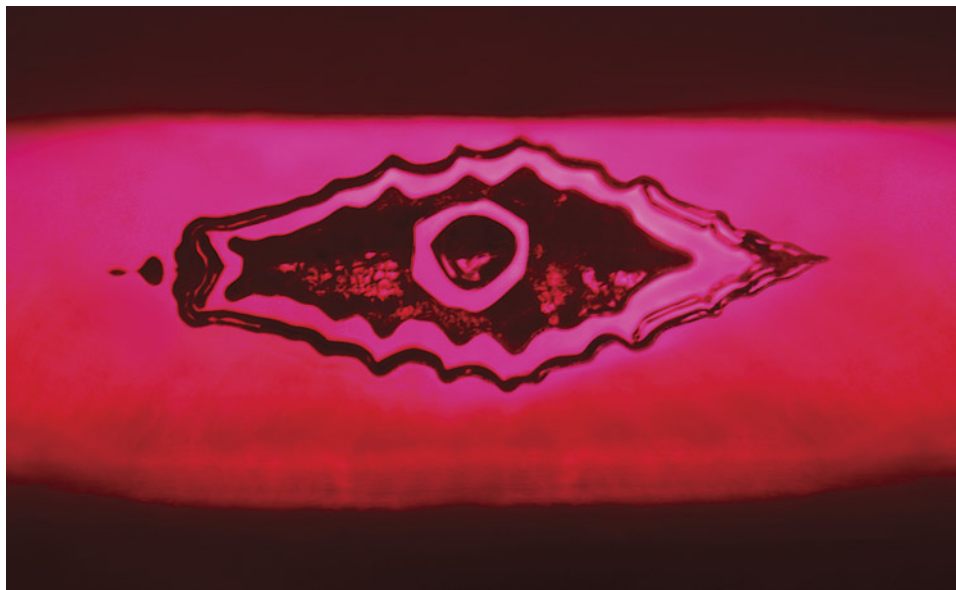
Figure 15. The reflection of a flux-healed fissure from a step pavilion facet in this Mong Hsu ruby resembles an evil eye. Photomicrograph by Ungkhana Atikarnsakul; field of view 1.07 mm.
