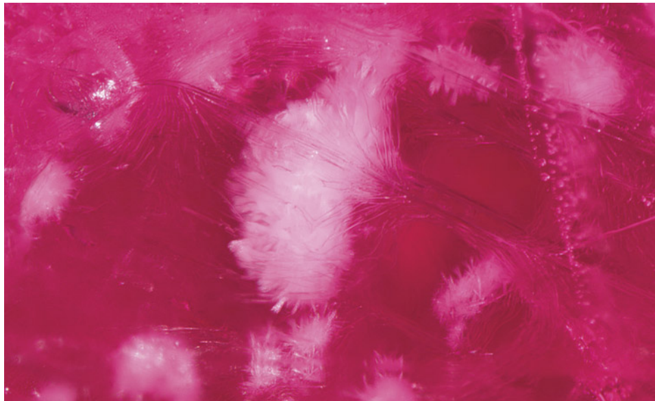
Figure 14. Devitrified glass inclusions resembling pom-poms or sea urchins in a clarity-enhanced ruby. Photomicrograph by Kevin Bishop and Joseph Hukins; field of view 1.99 mm.
