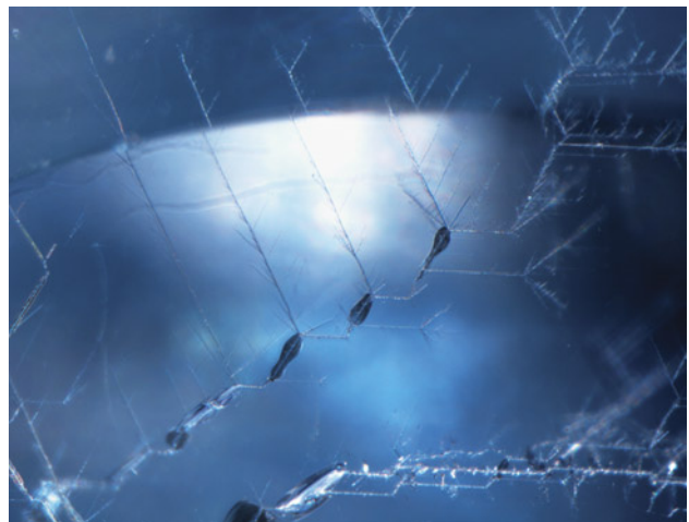
Figure 10. Hollow channels form unique patterns resembling a lightning strike in the 1.78 ct jeremejevite. Photomicrograph by Makoto Miura; field of view 1.06 mm.
