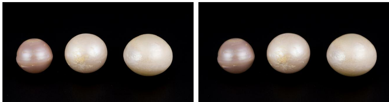
Figure 14. Pink Kasumiga pearls are shown before (left) and after (right) a fading test in these calibrated photos. The pearls were placed under a 100W tungsten lamp at less than 100°C for 30 minutes. The pink color has faded very slightly. Photos by Tetsuya Chikayama.
