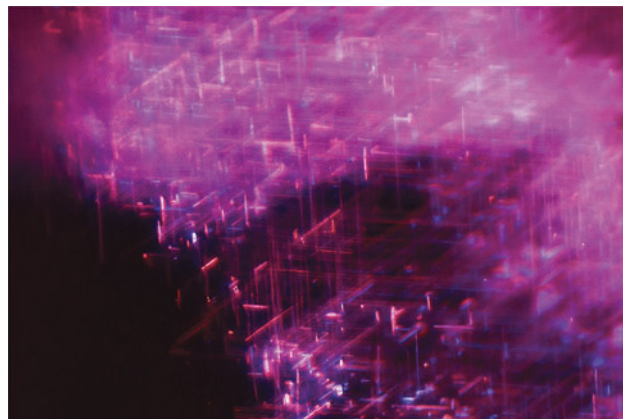
Figure 5. Dense, nested concentrations of silk in the ruby suggest an origin of Mogok, Myanmar. Photomicrograph by Huixin Zhao; field of view 1.13 mm.
