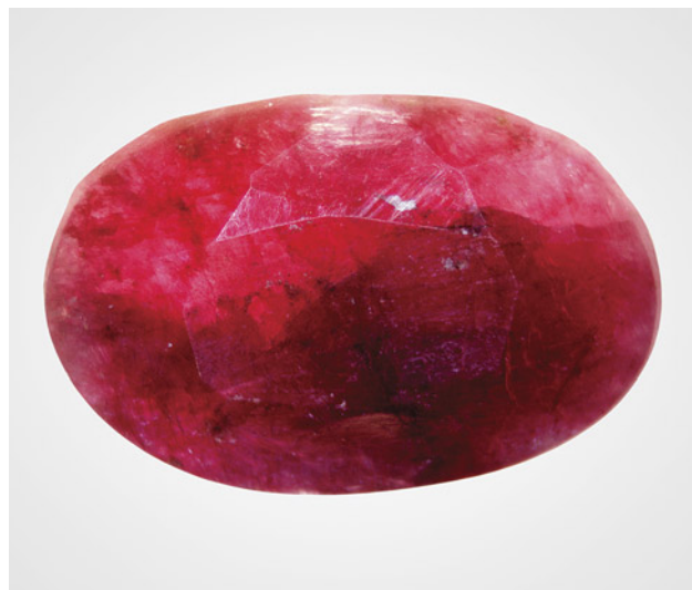
Figure 21. A semitranslucent 5.72 ct red-dyed spodumene, presented as “red corundum.” Photo by Guy Borenstein.
