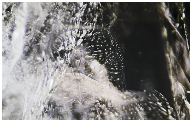
Figure 18. Magnification revealed obvious fluid and two-phase inclusions within the crystals. Photomicrograph by Lai Tai-An Gem Lab; field of view 4.60 mm.
