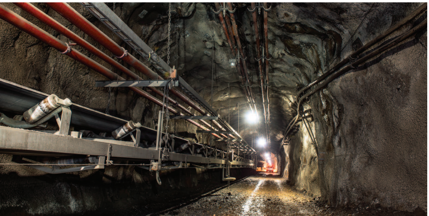
Figure 3. A recent view of underground operations at the Argyle mine, where 40 kilometers of tunneling have been built to access the diamond-bearing lamproite ore. Photo courtesy of Rio Tinto.
