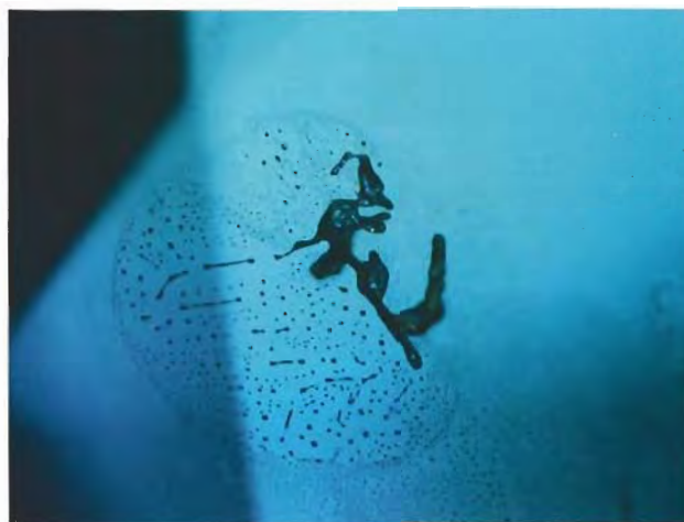
Figure 23. Heat treatment significantly altered the appearance of this group of crystals (zircon and uraninite!). They are shown here before (left) and after (right) the stone was treated. Photomicrographs © Rolf Schwieger; magnified 40 \times .
