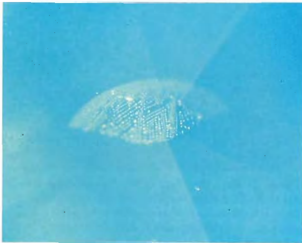
Figure 18. Fingerprint-like secondary healing planes were common in the Kashmir stones examined, but have also been found in sapphires from other localities. Photomicrograph © Rolf Schwieger; magnified 40×.
