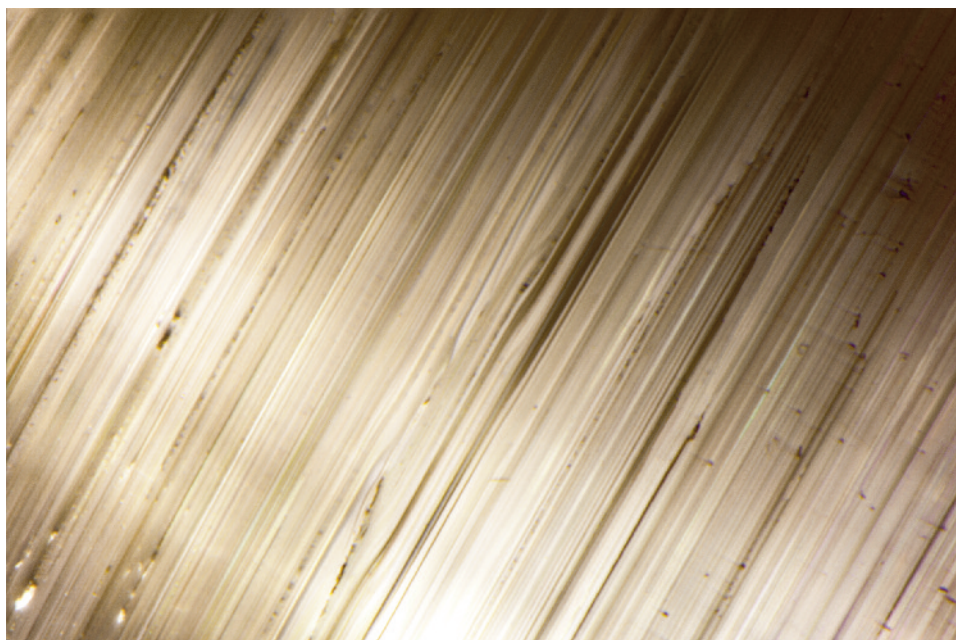
Figure 13. Growth tubes oriented along the c-axis and present only in the colorless portion are responsible for the chatoyancy in this bicolor tourmaline, observed using fiber-optic illumination. Field of view 3.59 mm. Photomicrograph by Nathan Renfro.
