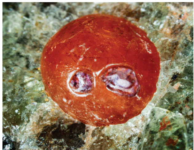
Figure 5. The larger inclusion in the apatite, a 5.74 mm sphere of orange calcite, featured a pair of purple “eyes” on its surface. Upon further analysis, these were revealed to be fluorite. Photomicrograph by John I. Koivula.
