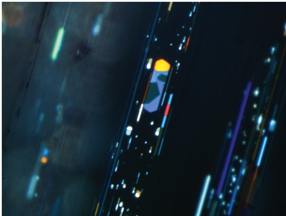
Figure 9. Viewed using oblique fiber-optic illumination, some of the iridescent platy voids in the phenakite contained complex multi-phase components consisting of a liquid, gas, and solid daughter crystals. Field of view 0.90 mm. Photomicrograph by John I. Koivula.
