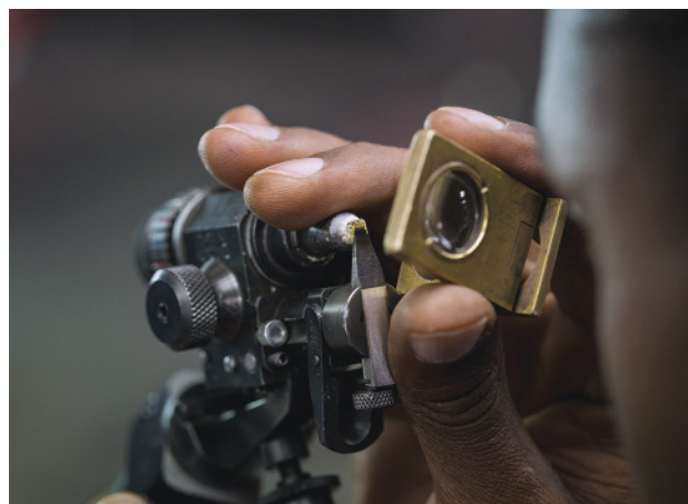
Figure 20. A cutter at Diacore Botswana examines the initial facets made on a fancy yellow diamond. Photo by Robert Weldon/GIA.
