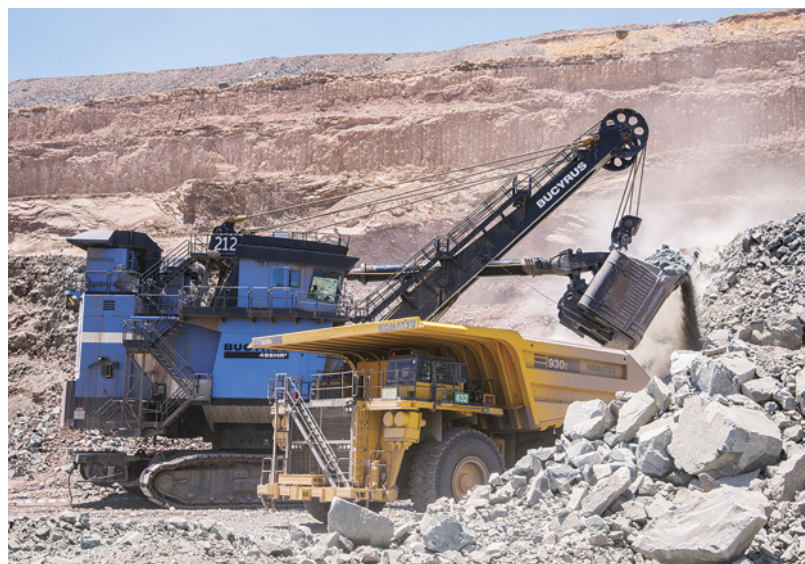
Figure 15. A Komatsu 930 truck can remove up to 250 tons of diamond-bearing rock and earth in a single haul. Photo by Robert Weldon/GIA.
