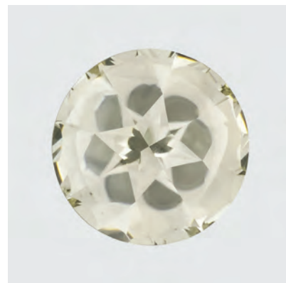
Figure 2. Viewed face-up, the buff-top diamond shows an arrangement of four main pavilion facets.
