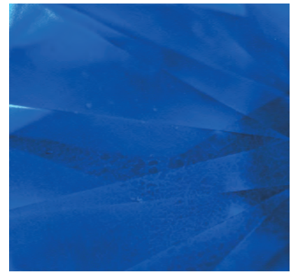
Figure 9. DiamondView imaging showed a micro-dislocation network on pavilion facets, conclusive proof of natural crystal growth.
