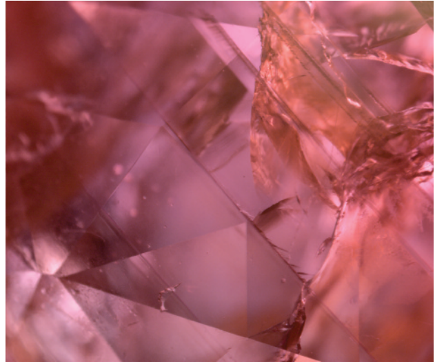
Figure 25. Contrasted twin lamellae in this ruby are similar to those often observed in material from Myanmar. Photomicrograph by A. Droux/LFG; magnified 60 \times .
