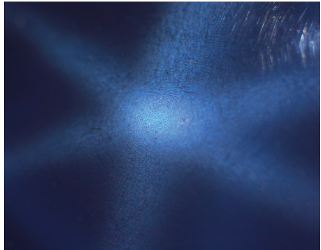
Figure 16. Very fine oriented needle-like inclusions causing the star were confined to a shallow layer below the surface. Photomicrograph by Sutas Singbamroong, magnified 25 \times .
