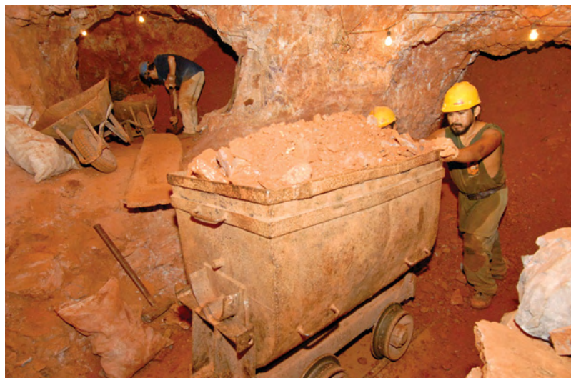
Figure 9. At Bolivia's Anahí mine, a worker removes an ore car loaded with quartz-bearing material that will then be washed and presorted. Photo by R. Weldon.
