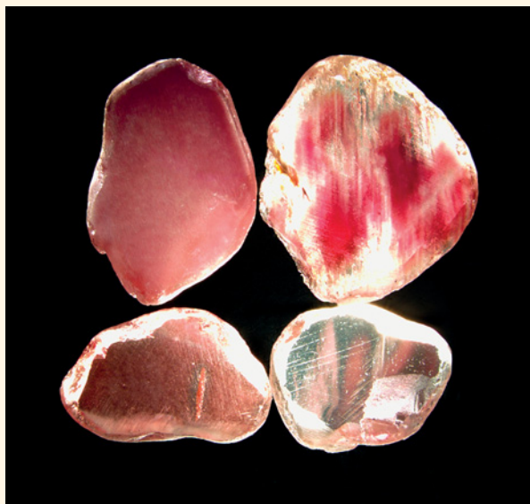
Figure 9. These Tibetan andesine samples (0.20–1.01 g, from Yu Lin Gu) show various uneven blue-green or red zones. Surface-reaching fractures are surrounded by narrow colorless areas. Photo by A. Abduriyim.
