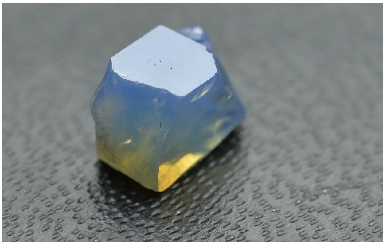
Figure 15: Tyndall effect in GIA reference sample 100309934811. The sample was placed on a black slightly reflective background and a white “daylight” type fluorescent illumination illuminated it from above. As can be seen blue color is scattered from the sides of the sample but when light reaches the lower part of the stone it becomes greenish and then yellow as most of the blue is scattered away. Photo: Vincent Pardieu © GIA.
