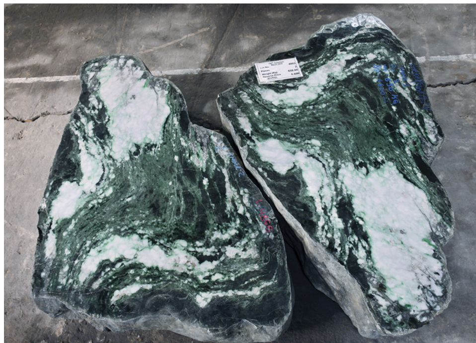
Figure 3. Sawn jadeite boulders, 650 kg total. Jadeite formed in ancient subduction zones where the circulation of fluids brought together all the necessary chemical components to form jadeite. These pieces clearly demonstrate the involvement of fluid flow in the formation of the jadeite. Photo by Wim Verriest.
