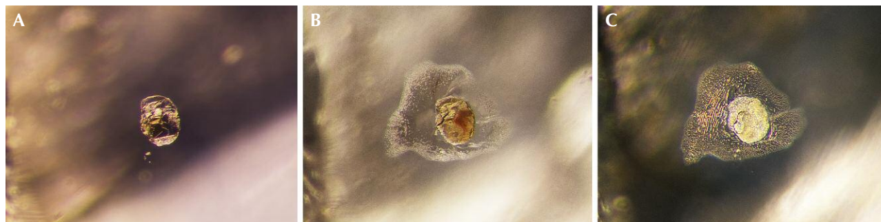
Figure 11. A: A small, flat crystal is pictured in sample 10 before heat treatment. B: A reflective fissure begins to appear around the crystal after the first heating to 800°C. By 1100°C (pictured), the fissure has begun to heal at the edges. C: By the last round of heating, at 1500°C, the fissure around this crystal has begun to heal into a fingerprint. The crystal itself has also changed and developed a frosty, whitish appearance. Darkfield illumination. Photomicrographs by E. Billie Hughes; field of view 1 mm.
