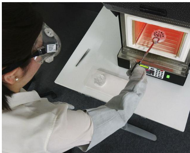
Figure 4. E. Billie Hughes removes the samples from the Vulcan 3-550 oven after a heating session. Photo by Rosey Perkins.
