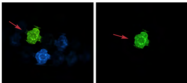
Figure 22. Left: The CVD-grown melee diamond (red arrow) shows green fluorescence in DiamondView imaging, while the natural melee below it exhibits blue fluorescence. Right: The DiamondView reveals the green phosphorescence of the synthetic melee, while the natural stone displays no phosphorescence. Images by Shi Tang.
