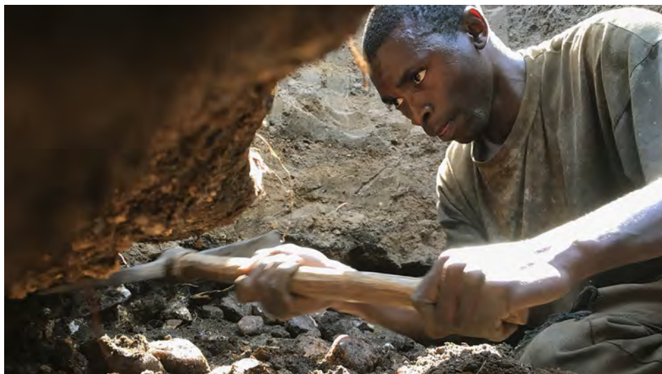
Figure 13. A garimpeiro working near the LP01 pit inside Mustang Resources’ concession near Napula village excavates the ruby-rich gravel under the topsoil. Photo by Vincent Pardieu.
