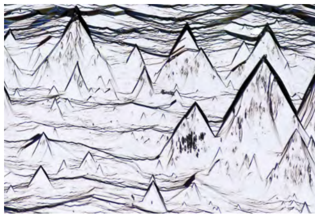
Figure 28. Differential interference contrast lighting reveals surface growth marks on Brazilian beryl. Photomicrograph by Jonathan Muyal; field of view 0.72 mm.
