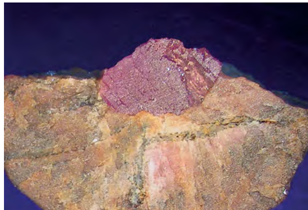
Figure 13. Rubies from secondary deposits at Tan Huong–Truc Lau are often coated by an iron-stained spinel aggregate. Here the spinel overgrowth has partially broken away from a ruby crystal (~2 cm across) after the specimen was sawn open. Photo by N. V. Nam.
