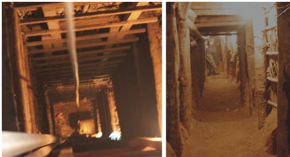
Figure 7. These photos show part of the shaft system of the Baw Mar mine (left) and horizontal development of the tunnel (right). Photos by Hpone-Phyo Kan-Nyunt.
