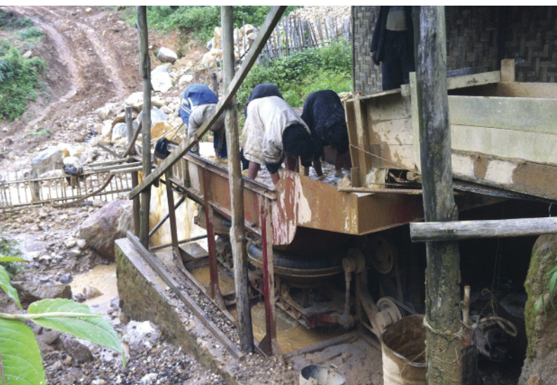
Figure 8. In this washing plant, gem gravel is concentrated and placed in drums. Photo by Daniel Nyfeler.
