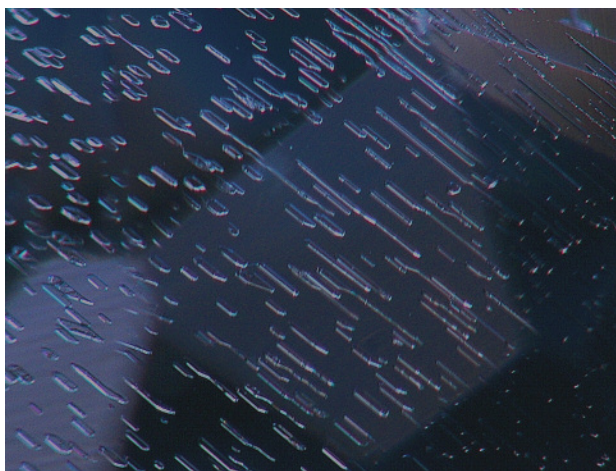
Figure 12. Healed fissure consisting of negative crystals in SABUM169. Photomicrograph by Hpone-Phyo Kan-Nyunt; magnified 25 \times .
