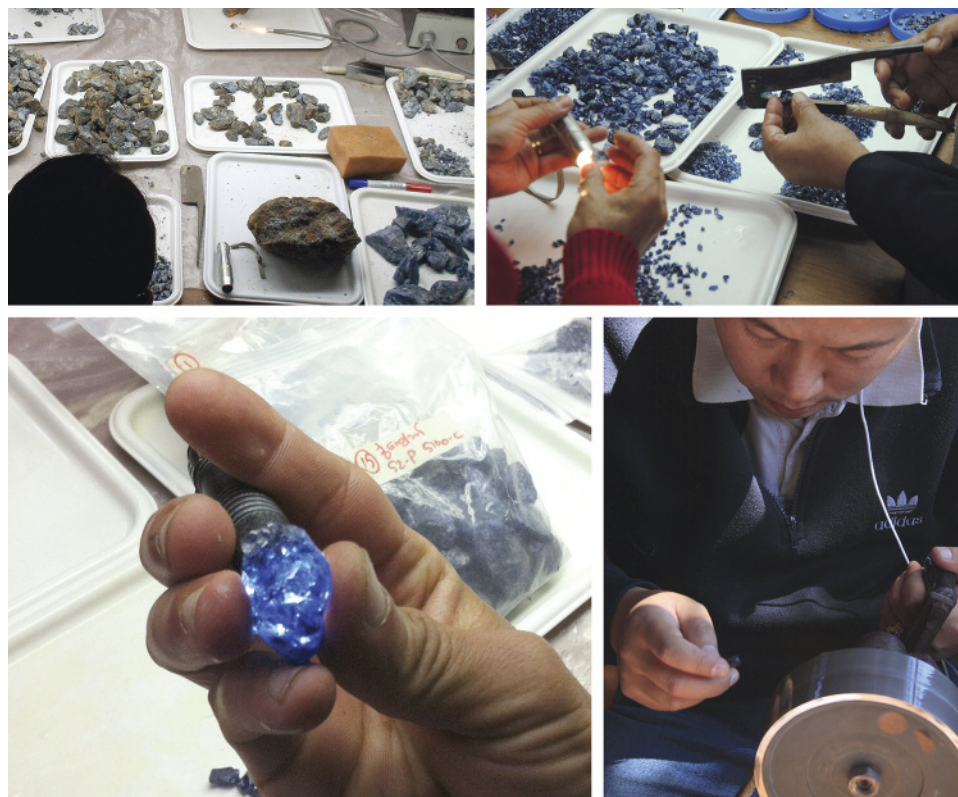
Figure 9. Top left: The sapphires from Baw Mar are sorted into different sizes and qualities. Some of the larger pieces can reach over 20 cm in length. Top right: The non-gem-quality portion of the rough is clipped off. Bottom left: After clipping, stones like the one here are left for faceting. Bottom right: Preforming sapphire from Baw Mar. Photos by Lore Kiefert (top left), Daniel Nyfeler (bottom left), and Hpone-Phyo Kan-Nyunt (top and bottom right).
