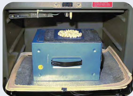
Figure A-3. The samples (here, a baroque strand ranging from 12.0 × 9.15 to 15.20 × 11.15 mm) are placed on the film immediately below the X-ray beam in the Faxitron unit. Photo by E. Schrader.
