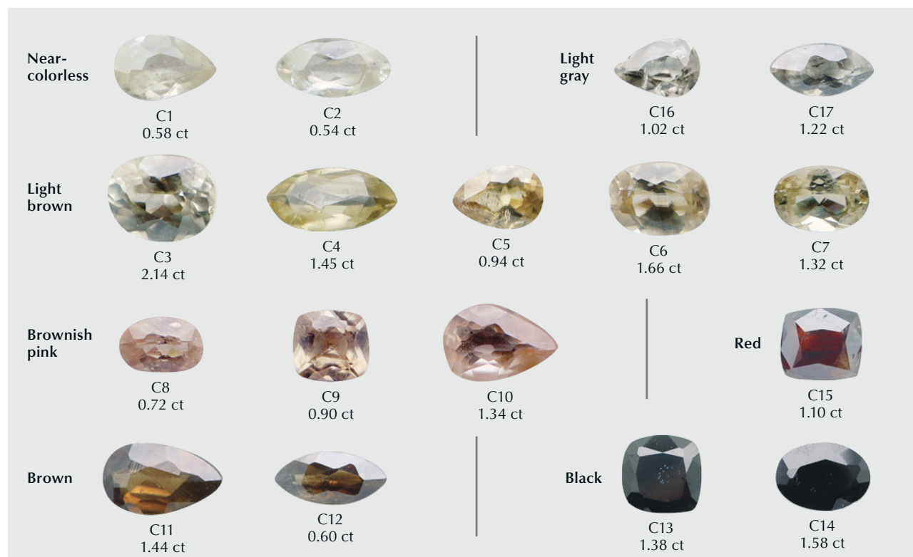
Figure 6. The 17 faceted cassiterite samples from the Yunling mine (0.54–2.14 ct) examined in this study. They represent the seven color groups of cassiterite from this deposit. Photos by Wenqing Huang.
