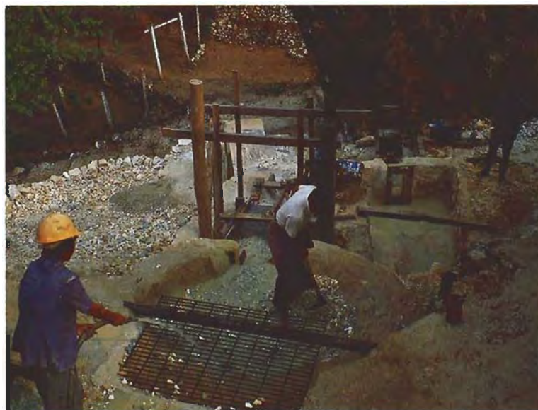
Figure 15. Just outside the entrance to the Lin Yaung Chi mine, the broken marble is passed through a series of screens. The large pieces are removed and sorted by hand in the screens on the left, while the smaller fragments continue downward through a series of sluices on the right, from which the gems are also recovered by hand. Photo by Robert C. Kammerling.
