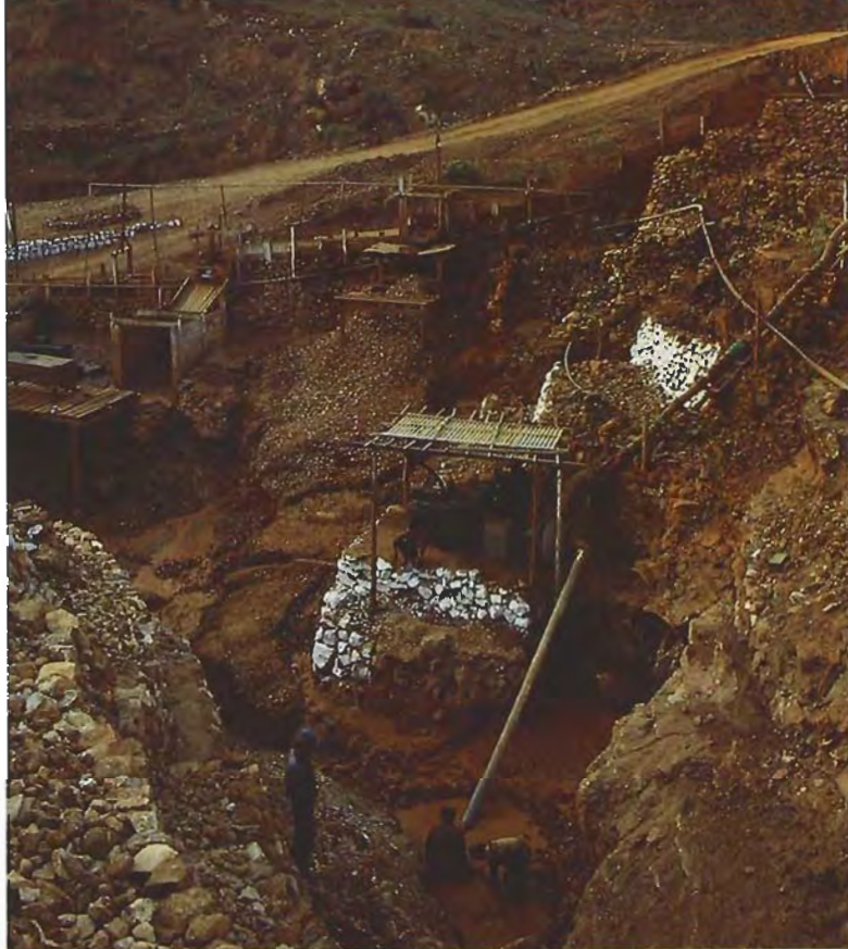
Figure 10. At a hmyawdwın, as shown here at the Yadanar Kaday-kadar mine, the water and gravel that are collected are subsequently pumped upward for processing. The gravels are then washed and large rocks removed before they are sent through a series of sluices (shown running diagonally at top center) in which the denser materials are trapped and hand sorted. Photo by Robert E. Kane.
