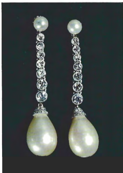
Figure 9. The two small pearls at the top of these earrings are natural, but the larger drops (approximately 10 × 14 mm) proved to be imitations made of solid glass coated with essence d'orient.
