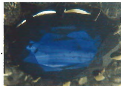
Figure 16. Two sets of curved color bands intersect in the wedge-shaped area at the center of this synthetic blue sapphire (7.5 \times 5.0 \times 3.1 mm). Magnified 10x.
