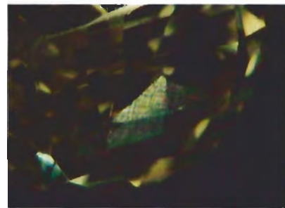
Figure 15. Plato lines characteristic of synthetic yellow sapphire were visible in this 6.93-ct stone even without magnification (shown here at 10x for clarity).
