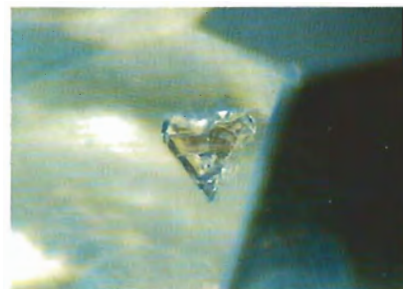
Figure 3. At 45 \times magnification, this heart-shaped inclusion is readily visible in the 13.08-ct host diamond.
