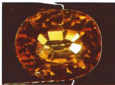
Figure 16. Dark yellow natural sapphire after heat treatment, reportedly not subject to fading. Magnified 10 \times .
