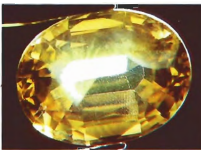
Figure 15. Light yellow natural sapphire after heat treatment. It was reported to be subject to fading. Magnified 12 \times .
