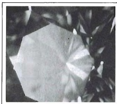
Figure 1. Irregular surface on the table of a diamond. Magnified 35 \times .
