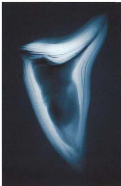
Figure 13. An X-radiograph of the pearl seen in figure 12 reveals the large hollow center characteristic of natural abalone pearls, surrounded by several layers of nacre, which is less transparent to X-rays.
