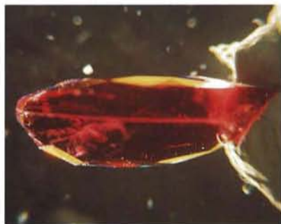
Figure 17. This profile view shows the separation plane of a ruby/ruby doublet. Immersion, magnified 17 \times .
