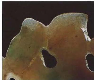
Figure 11. Magnification revealed not only that a piece at the top of the jadeite carving shown in figure 10 had been glued back on, but also that an adjacent area had been "reconstructed" with a polymer-like substance. Magnified 10 \times .
