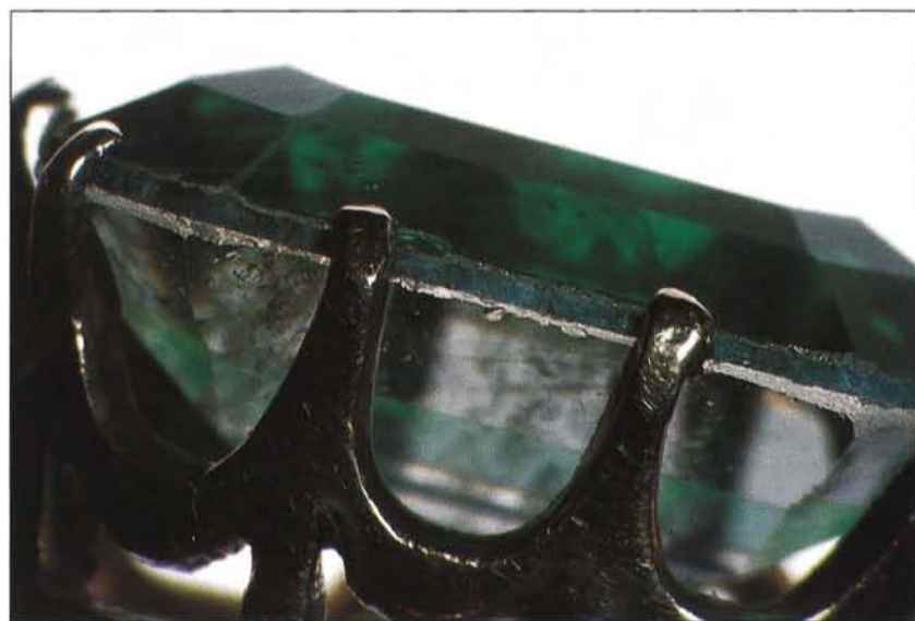
Figure 6. Magnification clearly reveals the separation plane at the girdle of the earring-set assembled stone shown on the left in figure 5. The green band in the pavilion is a reflection of the green cement at the girdle. Magnified 12×.
