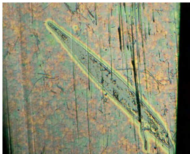
Figure 18. The pink surface coating on this topaz was easily scratched with a pin, as seen here in reflected light. Photomicrograph by Shane F. McClure; magnified 23×.
