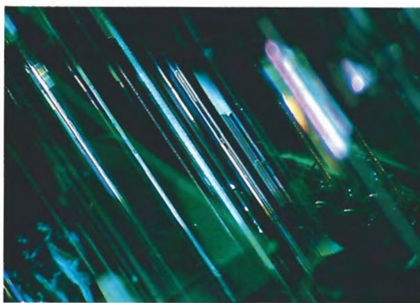
Figure 13. The growth tubes observed in the green tanzanites sometimes displayed interference colors. Photomicrograph by E. Boehm; magnified 30 \times .
