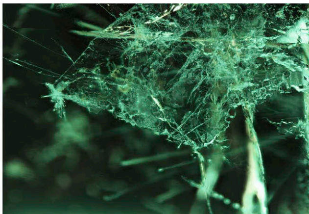
Figure 12. Left: The subtle luster difference reveals a relatively large quartz crystal inclusion and quartz veins breaking the table of the emerald host in reflected light. Right: The quartz crystal was also viewed in transmitted light, although less visible contrast was noted. Field of view (left and right) 7.19 mm.
