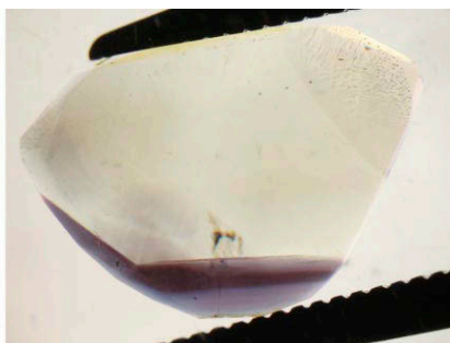
Figure 2. Viewed in immersion, the alexandrite displayed color zoning when viewed table-down (left) and from the side (right); field of view 12.5 mm.
