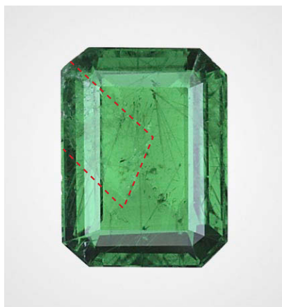
Figure 11. The red dashed line follows the edges of a large quartz crystal found breaking the surface of this 2.98 ct emerald.
