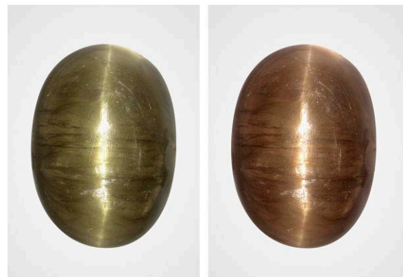
Figure 9. The 60.71 ct diaspore displaying color change and chatoyancy under fluorescent light (left) and incandescent light (right).
