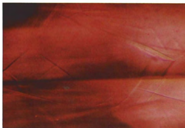
Figure 15. These curious swirl marks and growth features observed in Ghundao topaz appear to be connected to cleavage cracks. Such cracks in parallel alignment are an indication that these topazes should be treated with care. Magnified 30 \times .
