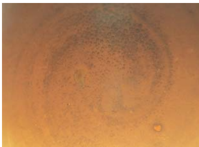
Figure 13. With 10× magnification, the imitation pearls shown in figure 12 exhibit gas bubbles and swirl marks below a smooth coating.
