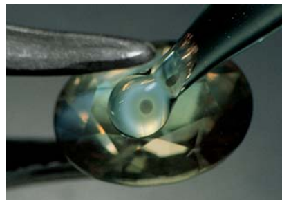
Figure 1. This unusual fish-eye effect was noted in a 2.93 ct alexandrite when it was observed in one particular direction through a condensing lens with cross-polarized light.
