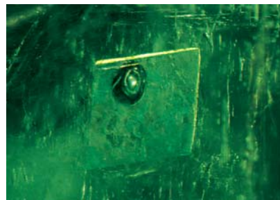
Figure 4. Note the prominent gas bubble and yellowish liquid filling in this rhombohedral void. As is typical of most large voids in such treated emeralds, the chamber is readily visible because the refractive index of the filler is sufficiently different from one or both of those of the surrounding emerald. Magnified 15 \times .
