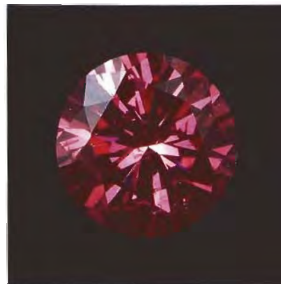
Figure 4. The color distribution in this 0.39-ct round brilliant is more even than that shown in figure 3. However, the diagnostic fluorescence and spectrum proved that the stone had been treated by irradiation and subsequent annealing.
