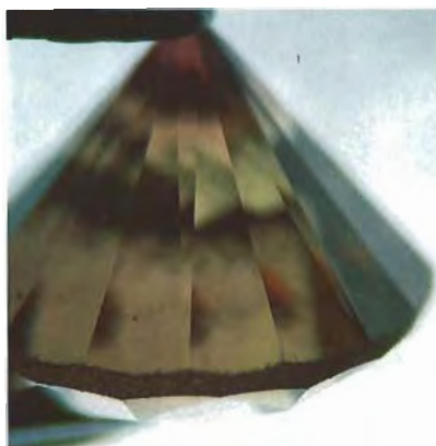
Figure 3. Uneven distribution of color, as illustrated by the pink and yellow zones in this 0.43-ct round brilliant diamond, is characteristic of treatment. Magnified 18 \times .
