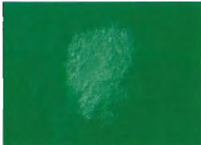
Figure 11. When we examined one of the jadeite cabochon's dark green inclusions in reflected light at higher (40×) magnification, we found that a less reflective substance was coating the boundaries between jadeite grains in the “inclusion” regions. (Because of the light scattering, this substance appears white in the microscope.)
