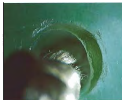
Figure 7. Residue of the polymer material with which this jadeite bead was impregnated is evident in its drill hole. Magnified 28×.
