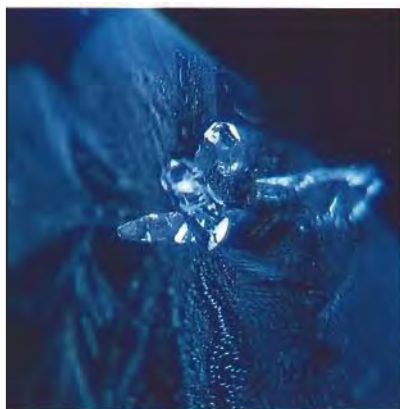
Figure 14. Seen magnified 63 \times at normal room temperature, these "crystal" inclusions in the blue sapphire shown in figures 11–13 lack stress fractures, which is key evidence that the stone had not been heat treated.
